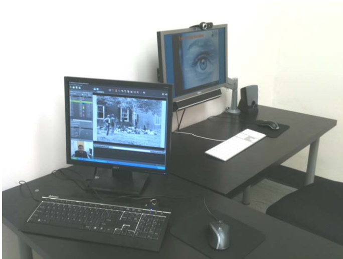
Fig. 2: Eye-tracking equipment in the Perception and Usability Testing Laboratory at Virginia Tech. An operator controls the foreground computer, and a subject sits in front of the screen in the back.
