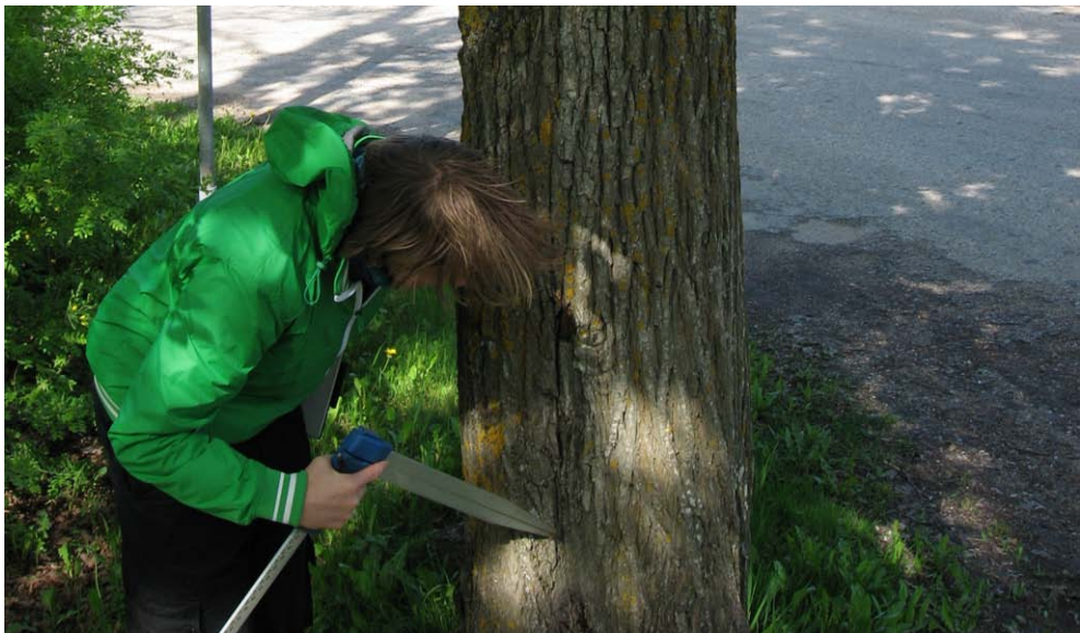
Fig. 1: Determining the damage on a tree trunk (Researcher is shown holding a calliper, a device for measuring trunk diameter)
