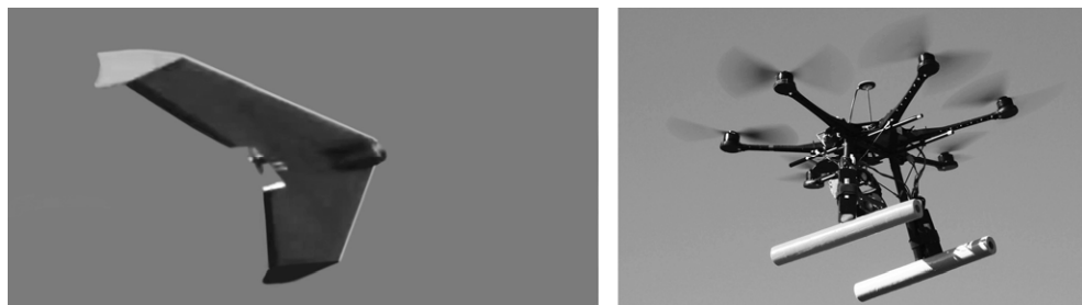
Fig. 1: RiteWingRC Zephyr flying wing and the DJI S800 hexacopter (Dr. Kevin Price)
