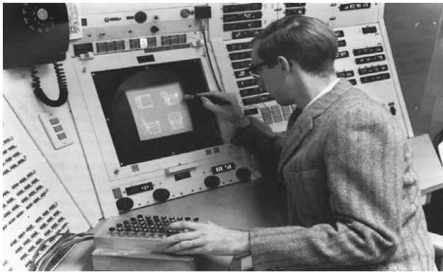
Fig. 8: Sketchpad developed beginning in 1961 by Ivan Sutherland at MIT is unveiled (Ref: Sutherland, Ivan E. Sketchpad: A Man-Machine Graphical Communication System. Proceedings of the AFIPS Spring Joint Computer Conference Washington, D.C., 1963, p. 329-346)
